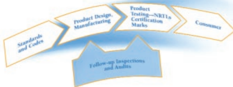
Figure 1. The Product Testing and Certification Process
